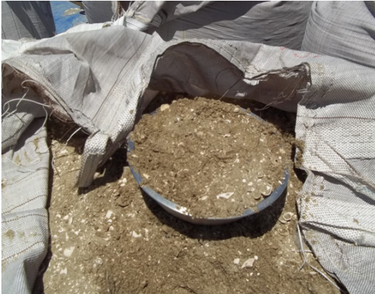
Figure 1. Sand material (mixed with shells) taken from trailing suction hopper dredger.
