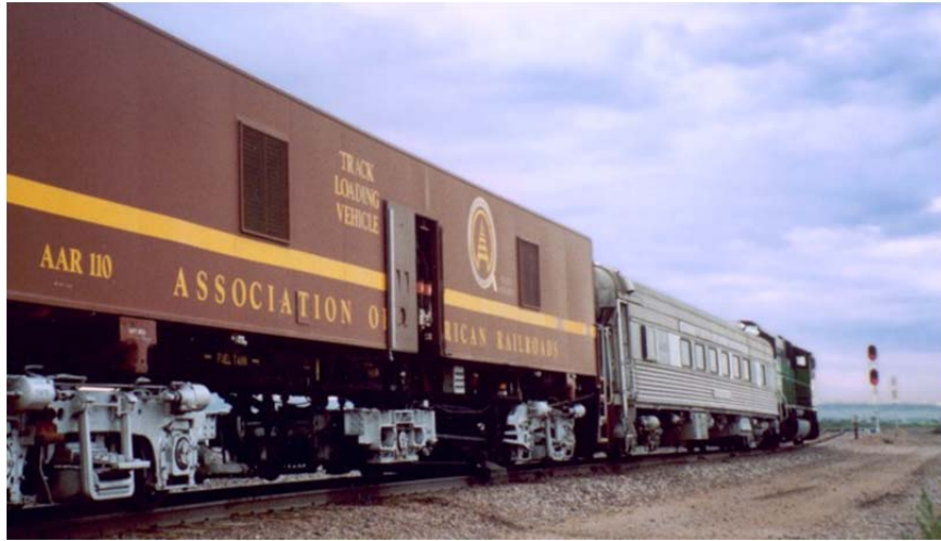
Figure 24: Track Loading Vehicle (TLV) at TTCI test track in Pueblo, Colorado (AAR)
