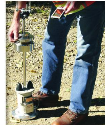
Several technologies for measuring the modulus of compacted geomaterials performed reasonably well, but lightweight deflectometers are recommended due to their ease of use and widespread availability.
