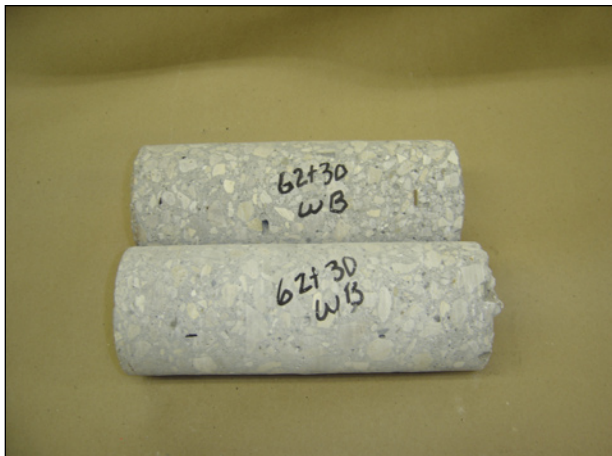
Figure 6. Core over the reflector plate (smooth bottom) and normal core (uneven bottom).
