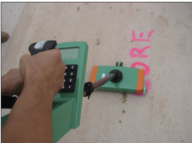
Figure 4. T2 located over the reflector plate.
