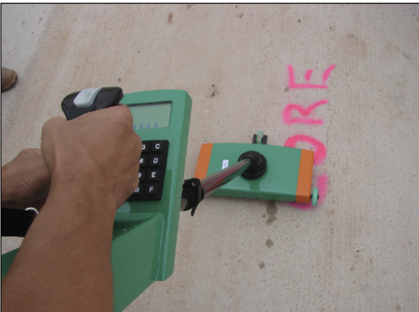
Figure 4. T2 located over the reflector plate.
