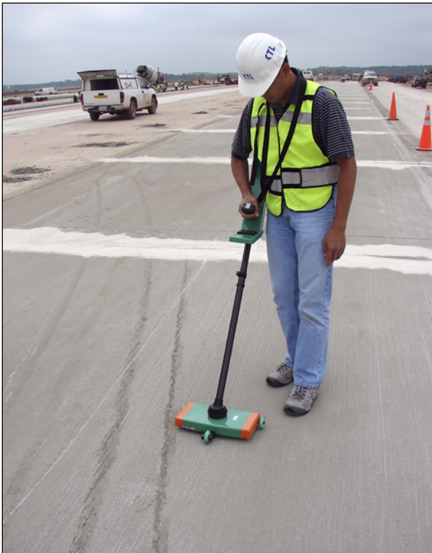
Figure 1. The MIT-SCAN-T2 device in use.
