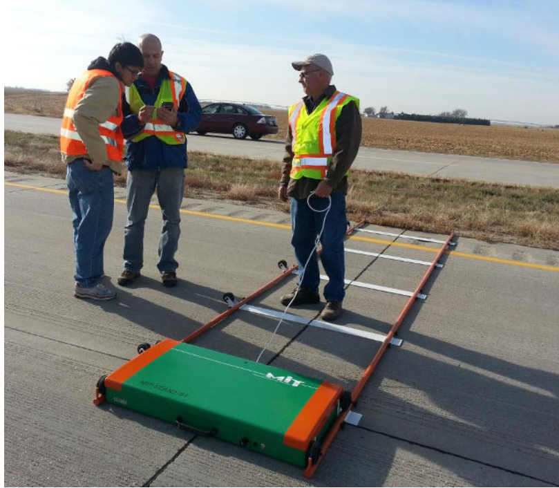
Figure 1.3 A joint being scanned by MIT Scan-2
