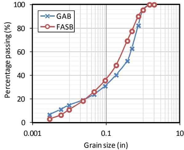
**Figure 2. Gradation of the GAB and FASB base materials.**
