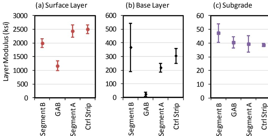
**Figure 7. Backcalculated moduli for the (a) HMA layer, (b) base layer, and (c) subgrade. Error bars indicate one standard deviation.**
