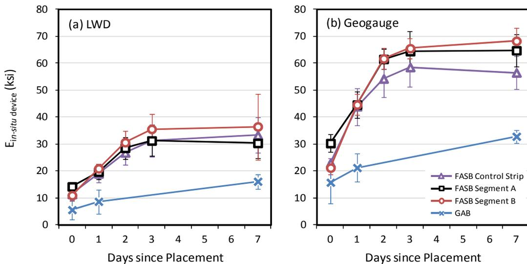
**Figure 5. The average stiffness increase with time as measured using (a) Zorn LWD, and (b) GeoGauge on FASB Control Strip, Segment A- second 4 inch lift, Segment B, and the companion GAB. Error bars show one standard deviation.**
