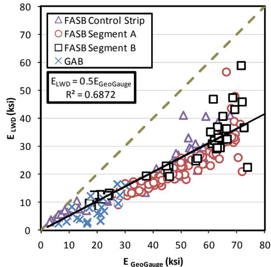
**Figure 3. Correlation between the stiffness measured by the Zorn LWD and GeoGauge on different FASB and GAB sections during 7 days of monitoring.**
