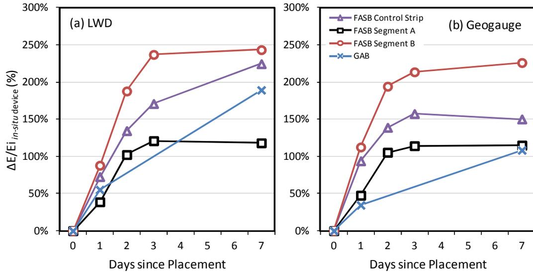
**Figure 6. The average percentage increase in stiffness as measured using (a) the Zorn LWD, and (b) GeoGauge on the FASB Control Strip, Segment A, Segment B, and the companion GAB. Error bars show one standard deviation.**
