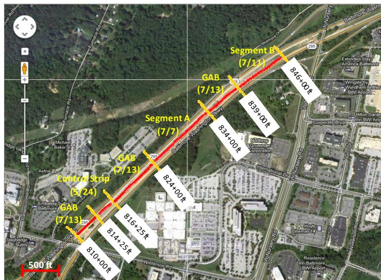
**Figure 1. Project plan. Numbers in parentheses indicate placement dates; numbers in white squares indicate the stations.**
