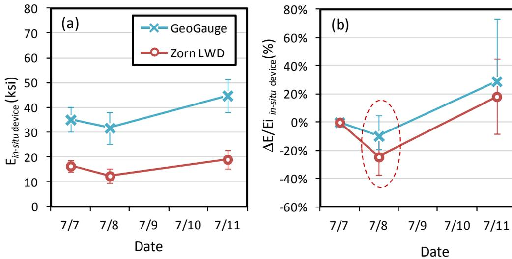
**Figure 4. The average (a) stiffness, (b) percentage increase in stiffness with time as measured using the Zorn LWD and GeoGauge on Segment A- first 4 inch lift.**
