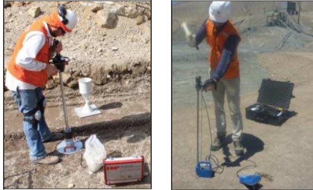
**Figure 1.** Dynamic lightweight plate LFG- Pro (left) and Dynamic lightweight penetrometer PANDA (right).
