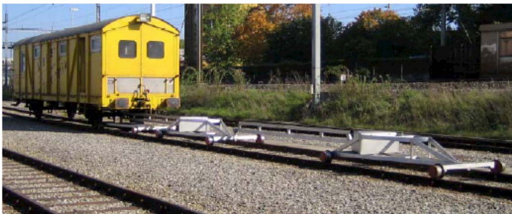
Figure 22: Swiss track stiffness measurement vehicle [17].
