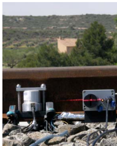
Figure 13: Geophone of 2 Hz and laser beam receiver clamped together to the rail base at the middle of a track span.
