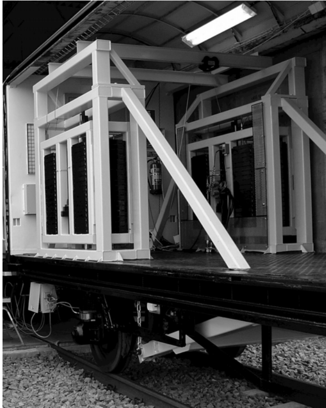
Figure 4. Photo of excitation equipment of RSMV
