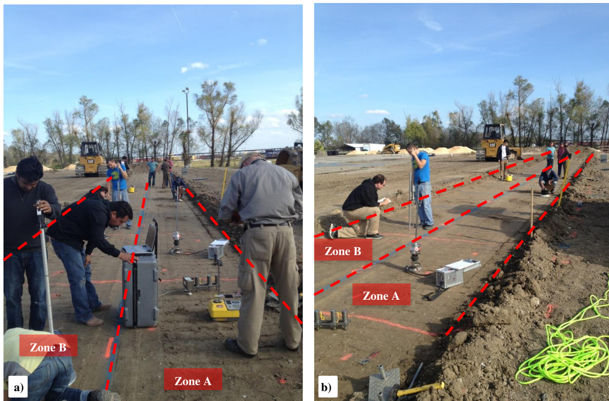
Figure G.2.5 – Nondestructive Testing of Compacted Pavement Layer at LTRC Test Sections
