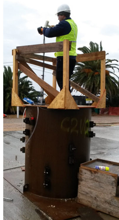
Figure 2. Execution of a Panda test on a chamber. The clamps at the outer side of the chamber are used to perform the vibrocompaction.
