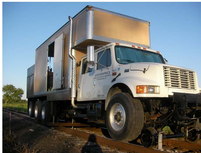
Figure 15: Stratigraphics CPT truck outfitted with High Railers performing penetration testing on an existing trackbed in Wisconsin (Stratigraphics)
