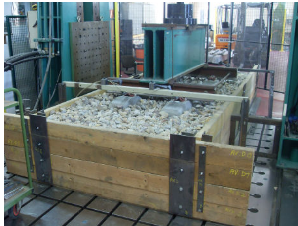
Figure 1: The full-scale track model used in this study
