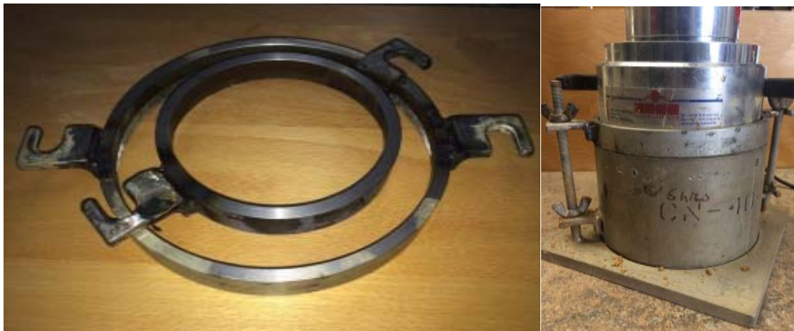
Figure 4-14. Attached collar during LWD on mold testing
