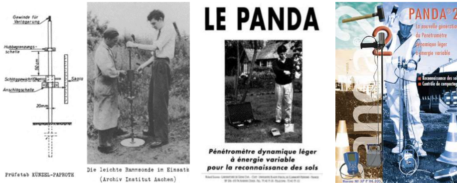
Figure 1. (a) Prüfstab Künzel-Paproth" (b) Panda® lightweight dynamic variable energy penetrometer: first generation and (c) Panda 2®: second generation.
