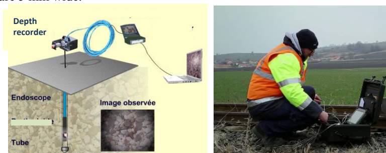
Figure 3: Geoendoscopy principle and photograph.
