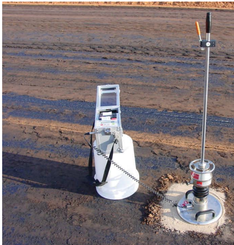
Figure 3: Portable Falling Weight Deflectometer
