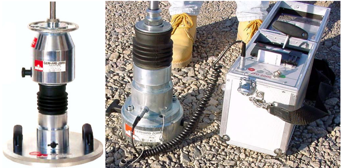
Figure 7: Alternative configurations of falling-weight deflectometer left: Medium-heavy falling-weight deflectometer using a 15 kg drop load and a load plate diameter of 300 mm. right: Medium-heavy falling-weight deflectometer with a load plate diameter of 150 mm.
