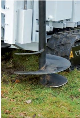
The Midi CPT Crawler consists of our proven HYSON 200 kN penetrometer mounted on an undercarriage with rubber tracks. The Midi CPT Crawler from A.P. van den Berg is designed to be compact, manoeuvrable and light, but with maximum power. With a weight of about 3,500 kilo and a width of only 1,200 mm the Midi CPT Crawler fits through small passages and can be transported in a small truck. All these features ensure that the crawler can be easily used, moved and transported.
