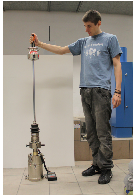
FIG. 3 Dynamic CBR test by using a falling weight LFWD to produce a defined load pulse of the CBR piston.
