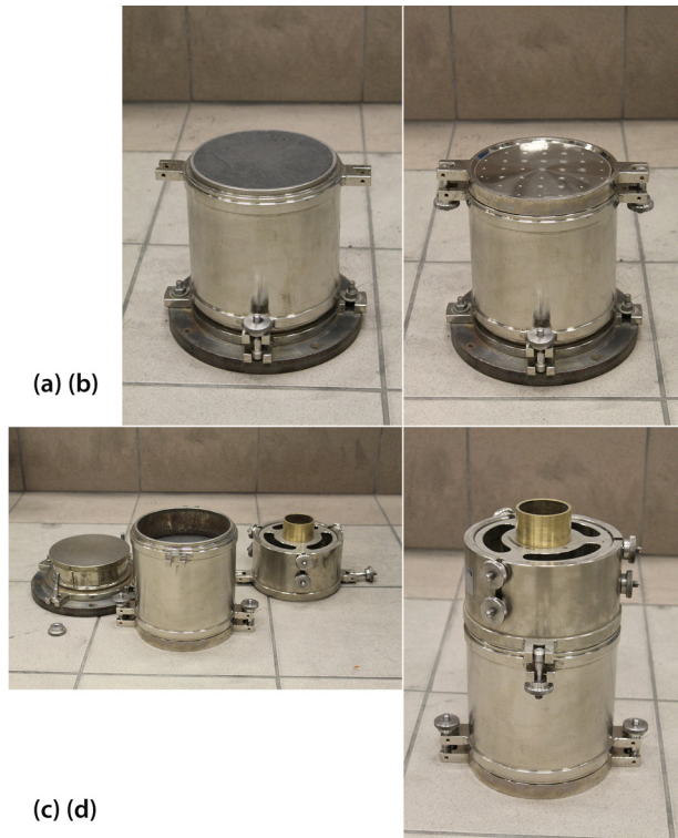
FIG. 2 Individual steps of preparing specimen for laboratory dynamic CBR test: (a) specimen after static CBR test and leveling surface, (b) mold with two bases for static (bottom) and dynamic (upper) tests, (c) specimen in mold with base for dynamic CBR before loading (on the left, base for static test, and on the right, mold extension to drive CBR piston), and (d) mold with extension ready for dynamic test.
