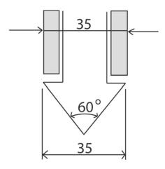
**Figure 3.** Early Dutch mechanical cone (after Sanglerat, 1972)
