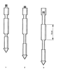
Figure 6. Begemann type cone with friction sleeve
