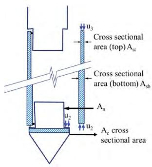
Figure 21. Unequal end area effects on cone tip and friction sleeve
