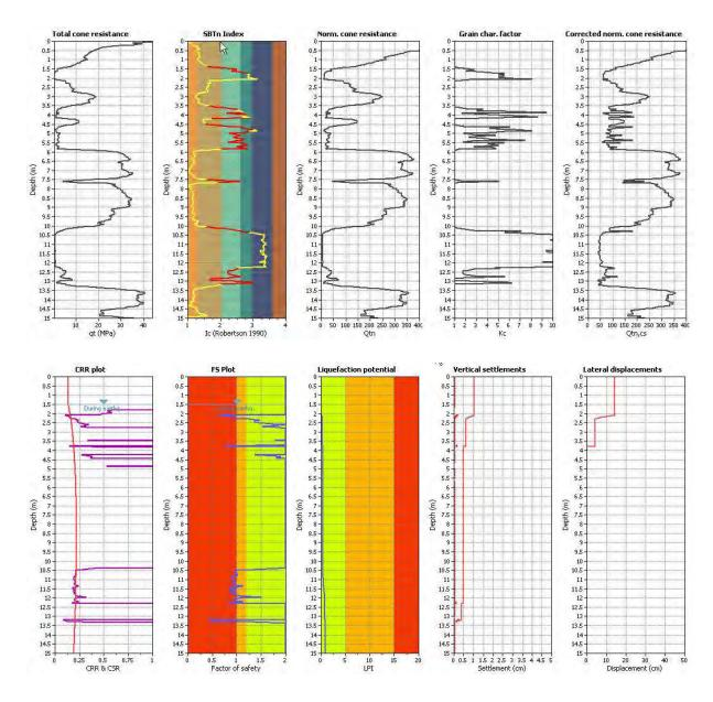
**Figure 53.** Example of CPT-based approach to evaluate cyclic liquefaction at Moss Landing Site showing (a) intermediate parameters (b) CRR, FS and post-earthquake deformations using '*CLiq*' software (http://www.geologismiki.gr/)
