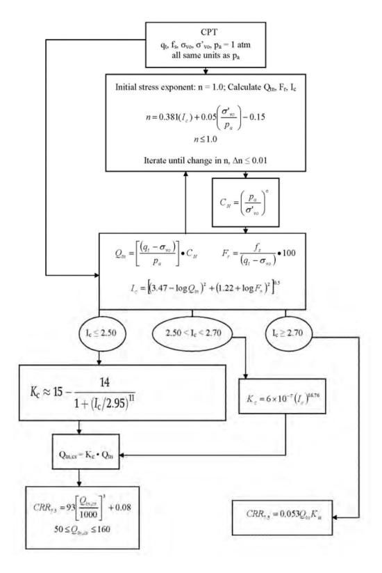
Figure 48. Flow chart to evaluate cyclic resistance ratio (CRR<sub>7.5</sub>) from CPT
