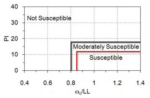
Figure 46. Liquefaction susceptibility criteria (after Bray and Sancio, 2006)
