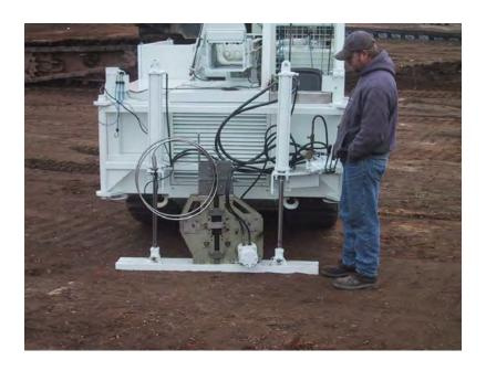
**Figure 14.** Mini CPT system with coiled rod delivery attached to small track mounted auger rig
