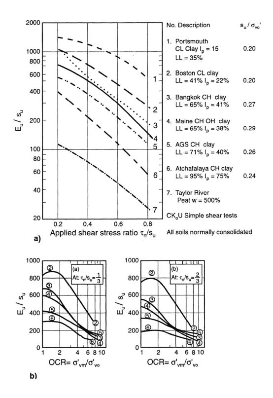
**Figure 42.** Selection of soil stiffness ratio for clays (after Ladd et al., 1977)
