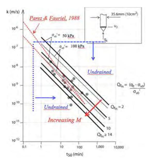
**Figure 35.** Relationship between CPTu  $t_{50}$  (in minutes), based on  $u_2$  pore pressure sensor location and  $10 \text{cm}^2$  cone, and soil permeability  $(k_h)$  as a function of normalized cone resistance,  $Q_{tn}$  (after Robertson 2010)
