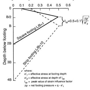
**Figure 39.** Strain influence method for footings on sand (Schmertmann, 1970)
