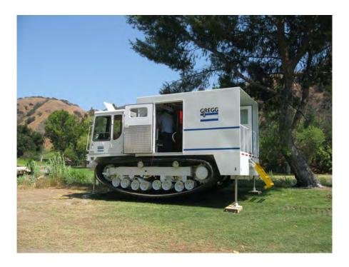
Figure 11. Track mounted 200kN (20 ton) CPT unit
