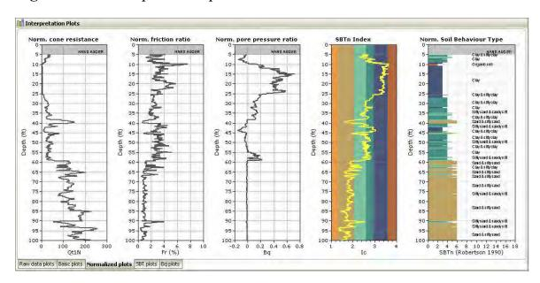
Figure 59. Example CPTu plot based on normalized parameters from *CPeT-IT*
