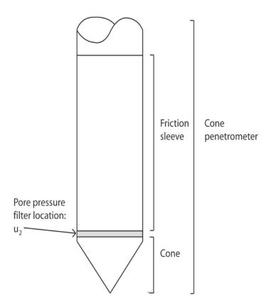
Figure 2. Terminology for cone penetrometers
