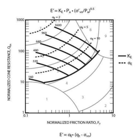
**Figure 40.** Evaluation of drained Young's modulus from CPT for uncemented sandy soils,  $E = \alpha_E(q_t - \sigma_{vo})$
