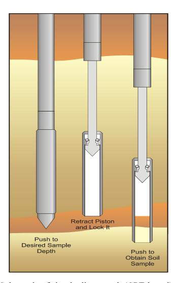
**Figure 1.** Schematic of simple direct-push (CPT-based) soil sampler (www.greggdrilling.com)
