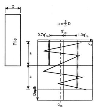
**Figure 43.** Calculation of equivalent average cone resistance (Bustamante and Gianeselli, 1982).
