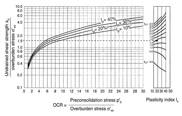
**Figure 29.** OCR and  $K_o$  from  $s_u/\sigma'_{vo}$  and Plasticity Index,  $I_p$  (after Andresen et al., 1979)
