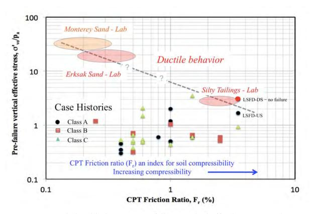
**Figure 56.** Relationship between pre-failure vertical effective stress and CPT normalized friction ratio for flow liquefaction case histories and selected laboratory results (After Robertson, 2017)
