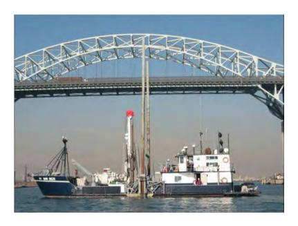
Figure 16. Quinn Delta (Gregg) ship with spuds
