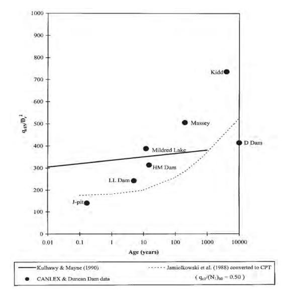
Figure 30. Effects of soil age on CPT penetration resistance in sands (note:  $q_{t1N} = Q_{tn}$ ) (After Fear et al. 2000)
