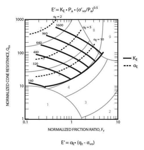
**Figure 32.** Evaluation of drained Young's modulus (at ~ 0.1% strain) from CPT for young, uncemented silica sands,  $E = \alpha_E(q_t - \sigma_{vo})$  where:  $\alpha_E = 0.015 \left[10^{(0.55Ic + 1.68)}\right]$
