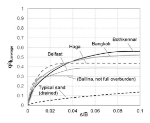
**Figure 38.** Field data for mobilized bearing stress vs settlement ratio (s/B) for footing on clay (Lehane (2017)
