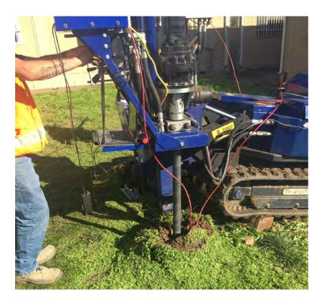
Figure 12. Small, anchored drill-rig unit
