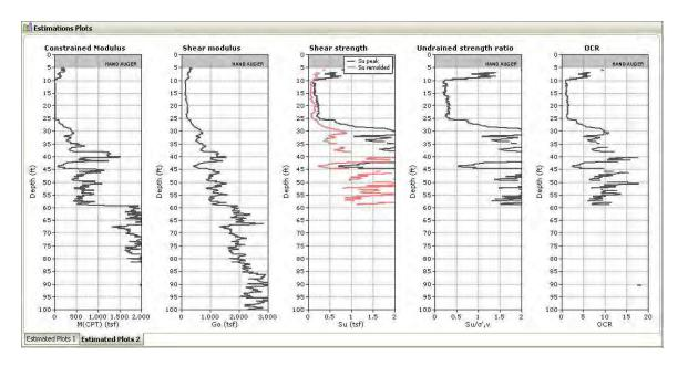
Figure 60. Example of estimated geotechnical parameters from CPeT-IT
