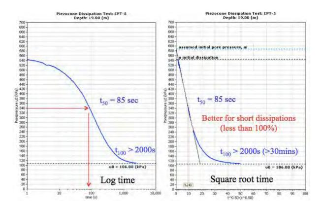
**Figure 19.** Example dissipation test to determine  $t_{50}$  and  $u_o$
