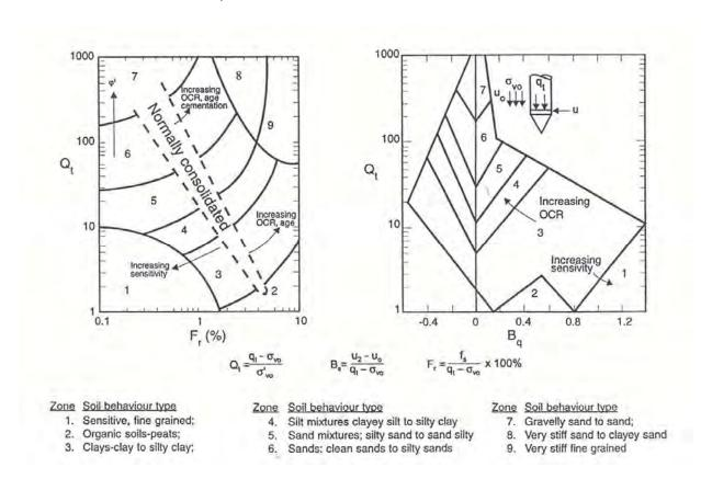
**Figure 24.** Normalized CPT Soil Behavior Type (SBT<sub>n</sub>) charts  $Q_t - F_r$  and  $Q_t - B_q$  (after Robertson, 1990).
