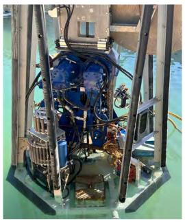
It is also possible to push the CPT from the bottom of a borehole using down-hole equipment. The advantage of down-hole CPT in a drilled borehole is that much
