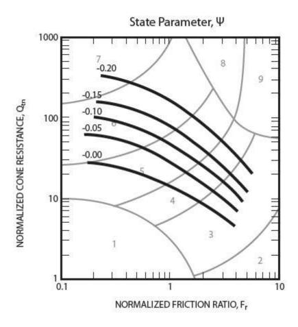
**Figure 31.** Contours of estimated state parameter,  $\psi$  (thick lines), on normalized SBT<sub>n</sub> Q<sub>tn</sub> – F<sub>r</sub> chart for uncemented Holocene-age soils (After Robertson, 2009)
