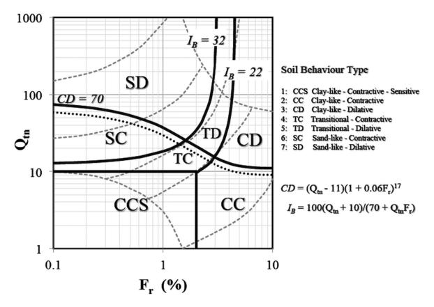
**Figure 25 (b).** Updated Normalized CPT Soil Behavior Type (SBT<sub>n</sub>) O<sub>tn</sub>-F<sub>r</sub> chart (After Robertson, 2016)
