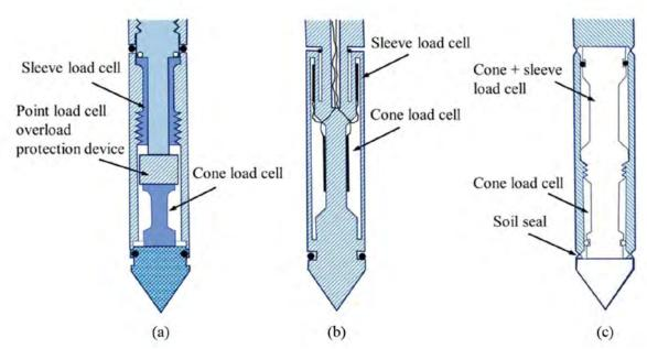
**Figure 20.** Designs for cone penetrometers (a) tip and sleeve load cells in compression, (b) tip load cell in compression and sleeve load cell in tension, (c) subtraction type load cell design (modified from Lunne et al., 1997)
