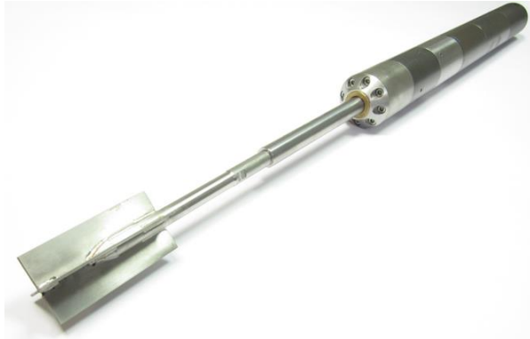
Figure 1. The A.P. van den Berg Icone Vane (without protection tube).
