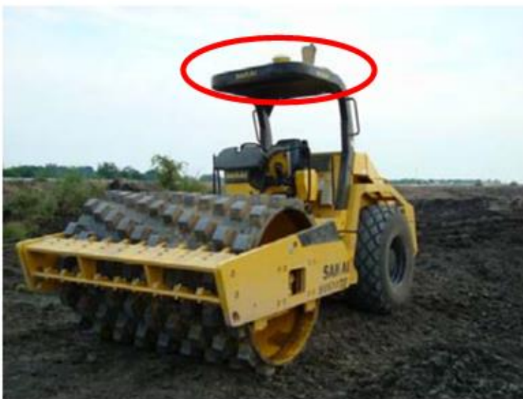
Figure 2.2 Real-time kinematic GPS receiver and antenna on a Sakai roller ( White & Vennapusa 2010)
