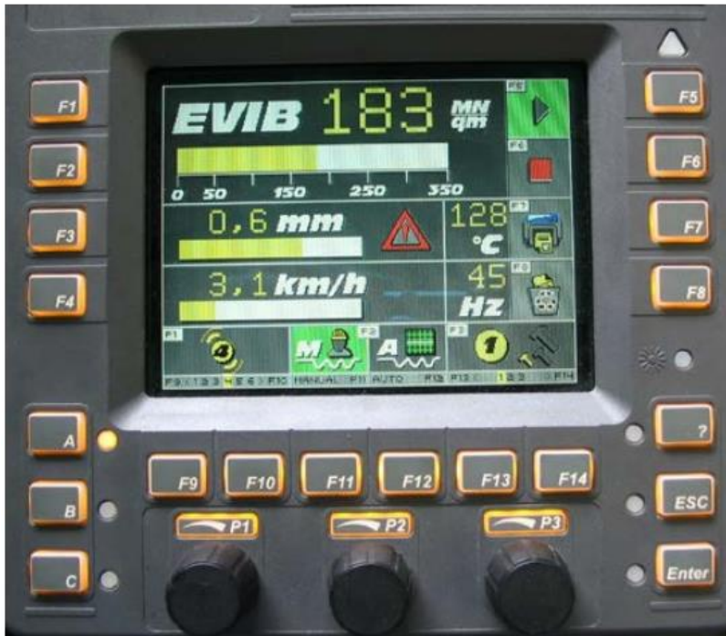
Figure 4.3 Bomag IC on board display (Chang et al. 2011)
