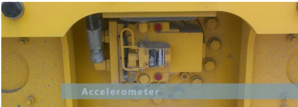
Figure 2.1 Accelerometer sensor mounted on the roller frame (Nieves 2014)
