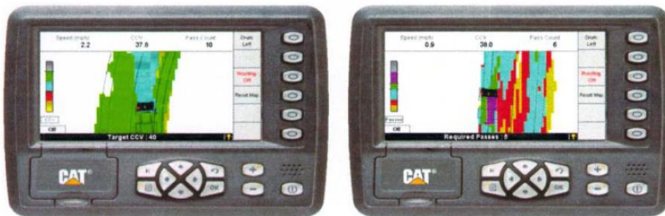
Figure 2.3 Caterpillar documentation system illustrating completed passes (left) and CMV (right) (Mooney et al. 2010)
