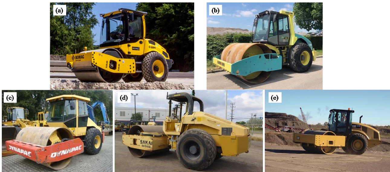
Figure 4.1 Pictures of different rollers used for intelligent compaction (a) Sakai (b) Ammann (c) Dynapac (d) Sakai (e) Caterpillar smooth-drum rollers (adapted from Chang et al. (2011))
