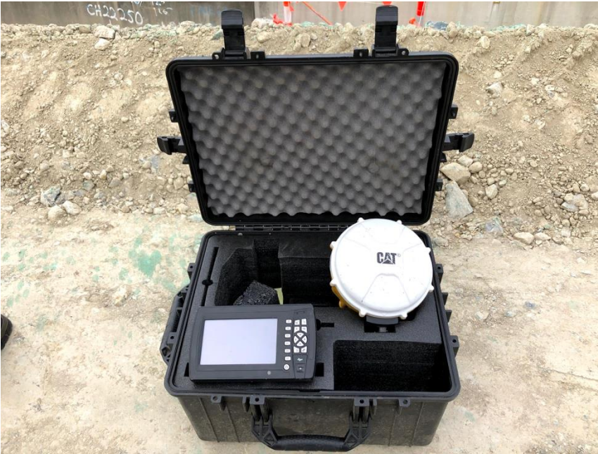
Figure 3.1 A Trimble intelligent compaction retrofit kit
