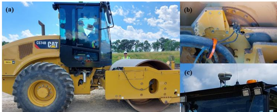
Fig. 1. (a) Caterpillar Vibratory Roller Fitted with (b) Accelerometers and (c) GPS
