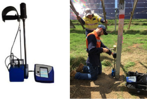
Figure 2. PANDA DCP (dynamic cone penetrometer)
