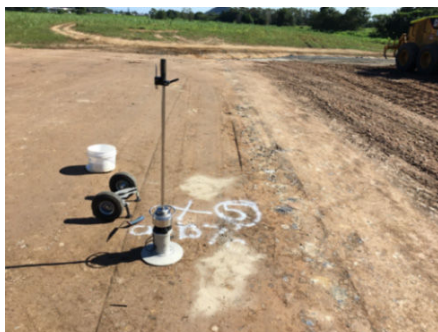
Figure 8. A density “pass” with a fail LFWD disagreement area
