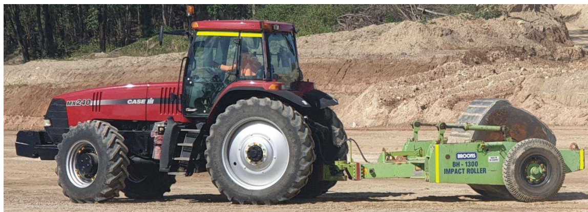
Figure 1: The 4-sided or “square” impact roller, with tow tractor
